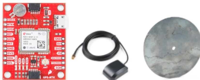
Figure 57: SparkFun NEO-M8P-2 Qwiic . Includes the Board, Base plate, and Antenna. Dimensions (in): 1.6 x 1.3 x 0.2, Mass (lb): 0.01. 32
