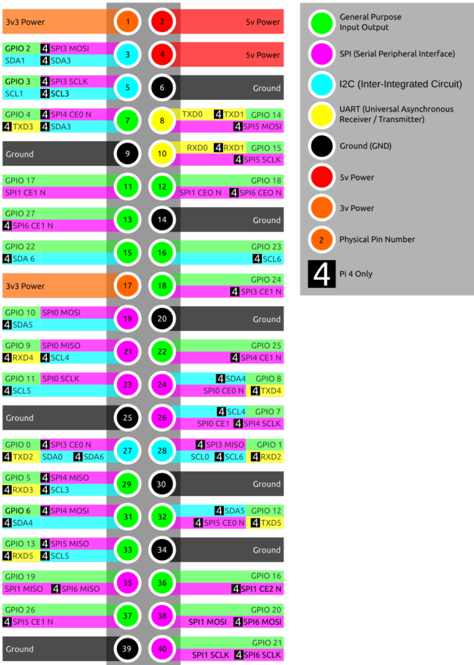
Figure A2: Raspberry Pi 4 Model B Pinout. This shows which pins can be used for I2C, UART, and SPI. Pins 12, 32, 33, and 35 are also capable of PWM. 47 48
